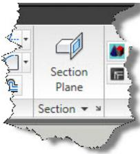
In order to create a cross section, you must first create a section plane, which you can do by using the Section Plane tool in the Section panel of the Home ribbon tab (when working in the 3D Modeling workspace). Note that these tools are also available in the Section panel on the Mesh Modeling ribbon tab.
